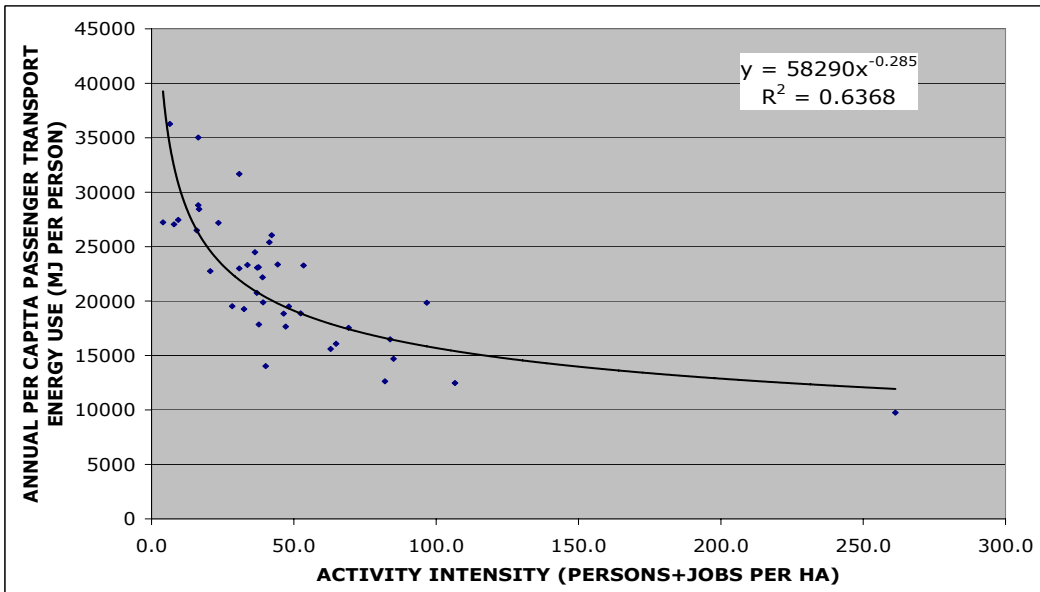
Figure 4. Per Capita Passenger Transport Energy Use versus Activity Intensity in Sydney Local Government Areas, 1981
